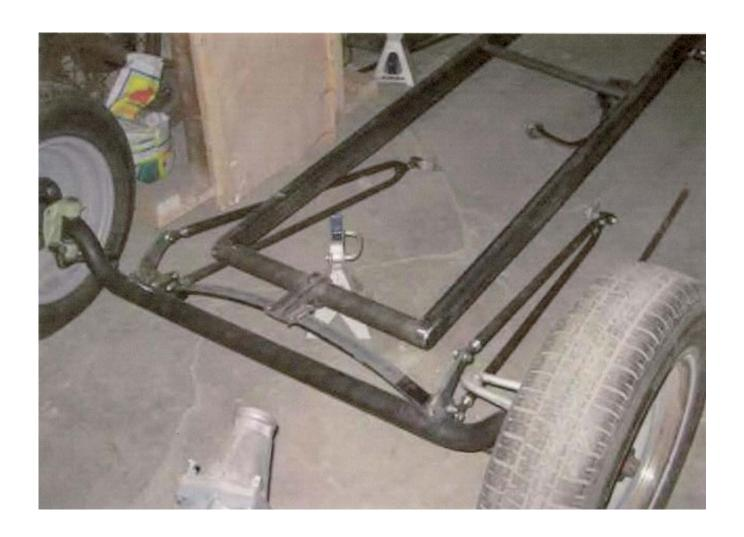
This packet is about setting up your rear suspension. The references to the rear axle are for an 8" Ford out of a Maverick. If you are using something else, you might have to make some adjustments to the given measurements and brackets.
